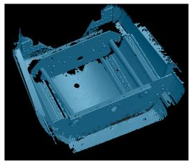
Three dimensional scan results include all of the critical details like the clearance for structure and contour of the fuselage. Also included are hole centerpoints to utilize existing mounting options.
