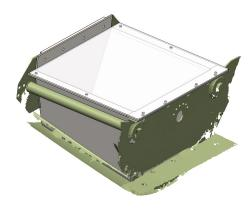
The scan reference provides excellent, accurate and detailed reference for generating a CAD model for fabrication of a steel container for lead weight.
