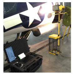
Utilizing portable hand-held 3D scanning allows for scanning on-site and easily reaching inside of hatches.
