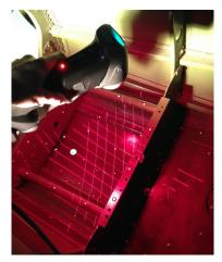
The seven lasers emitted from the scanner generate 480,000 measurements per second over the targeted area.
