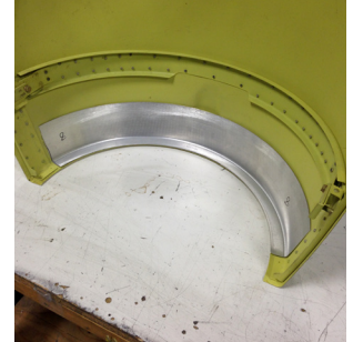
One half of the fabricated doubler located and reflecting it's perfect fit.
