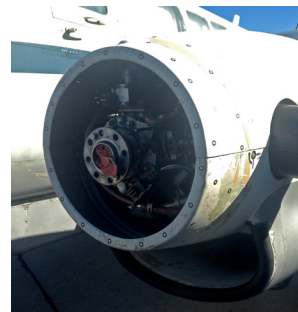
An existing cowl was used as the scanning subject. Note the scan was even performed on the ramp.
